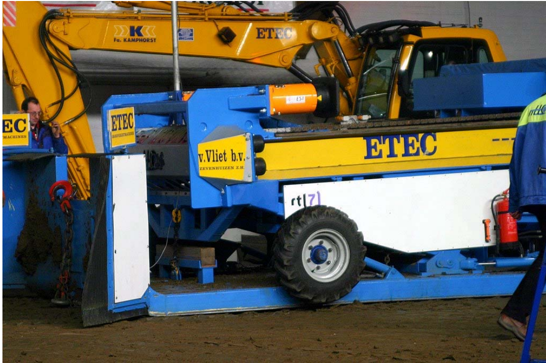
After modification to comply with the 2008 specifications. Please note the angle of the box rails and the buffers.
